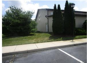
Parking spaces in the parking lot to the east of the building can be converted to porous pavement to capture and infiltrate stormwater runoff from the parking lot. A rain garden can be installed to the northwest of the building to capture, treat, and infiltrate stormwater runoff from the roof. A preliminary soil assessment suggests that more soil testing would be required before determining the soil's suitability for green infrastructure.
